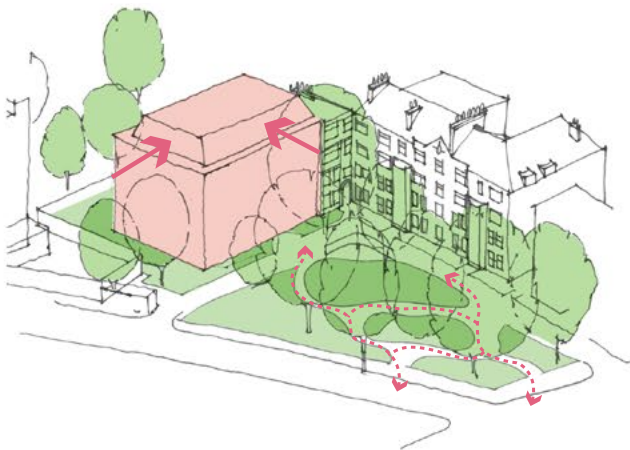
3. Set back top storey to create mansard roof. Open up access from Colehill Lane and enhance permeability across ornamental gardens.
