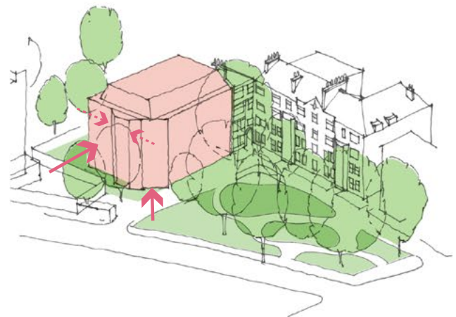
4. Chamfer edges to soften the corners and create a projecting bay stylistic of contextual Victorian houses.
